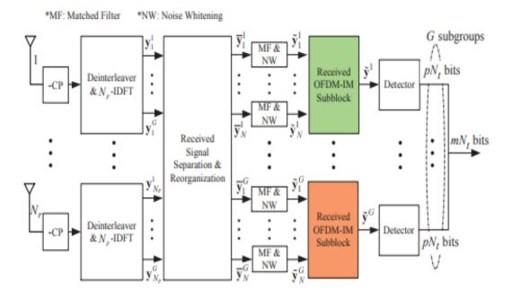
Fig. 2. Block diagram of MIMO-OFDM-IM receiver.
