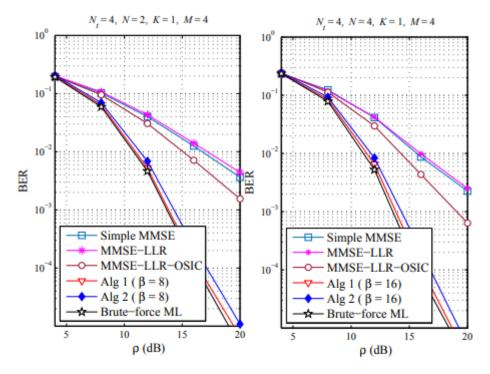
Fig. 3. BER performance comparison of different detection algorithms for MIMO-OFDM-IM with Nt = 4, K = 1, and QPSK modulation
