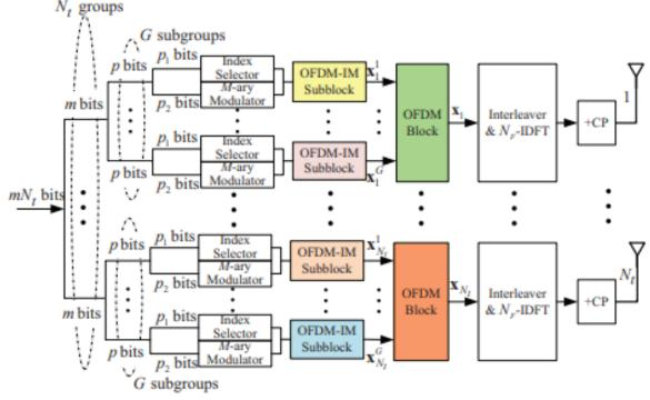
Fig. 1. Block diagram of MIMO-OFDM-IM transmitter.
